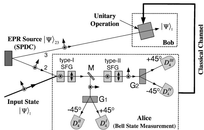
FIG. 1. Principle schematic of quantum teleportation with a complete BSM. Nonlinear interactions (SFG) are used to perform the BSM.  $\odot$  and  $\uparrow$  represent the respective horizontal and vertical orientations of the optic axes of the crystals.
