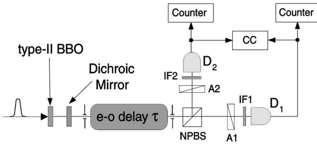
FIG. 1. The experimental setup. Type-II SPDC is separated from the residual UV pump beam by using a dichroic mirror. A pinhole selects the collinear SPDC. The coincidence counting rates are monitored as a function of the e-o delay  $\tau$ . See text for details.
