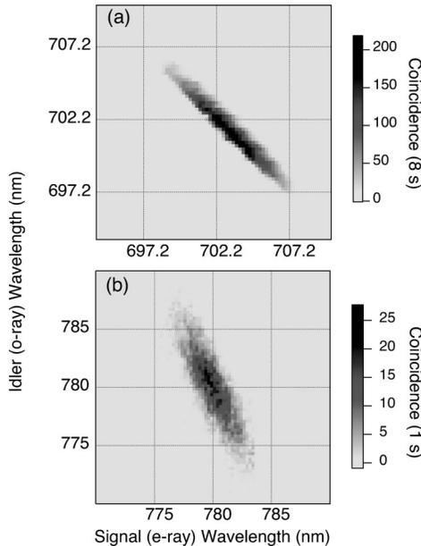
Fig. 4. Joint spectrum of type II SPDC for (a) cw UV pumping and (b) ultrafast UV pumping. The data are in good agreement with the theory plots shown in Fig. 1.
