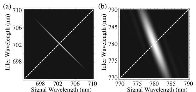
Fig. 1. Calculated joint spectrum functions for type II SPDC: (a) cw UV pumping and (b) ultrafast UV pumping. Dashed lines represent lines with the signal wavelengths equal to the idler wavelengths. Note the asymmetry in (b).
