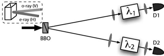
Fig. 2. Experimental setup: beamlike type II SPDC is used.  $\lambda_1$  and  $\lambda_2$  are monochromators.
