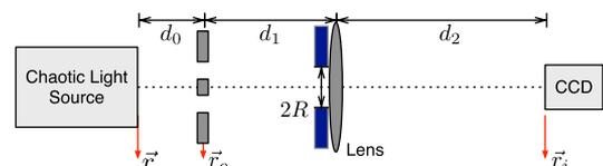
Fig. 1. (Color online) Conceptual scheme for sub-Rayleigh imaging via speckle illumination. See text for details.
