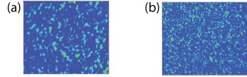
Fig. 3. (Color online) Speckle illumination with different transverse coherence  $l_c$  observed at the image plane through the fully open iris. (a)  $l_c = 119$   $\mu\text{m}$ . (b)  $l_c = 63$   $\mu\text{m}$ .
