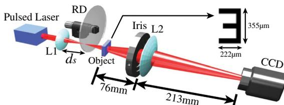
Fig. 2. (Color online) Experiment setup. Inset shows the object mask used in the experiment. See text for details.
