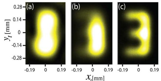
Fig. 4. (Color online) (a) Conventional intensity imaging. Image cannot be resolved. (b) and (c) Second-order correlation measurement with, respectively, speckle illumination shown in Figs. 3(a) and 3(b). Sub-Rayleigh imaging is clearly demonstrated.
