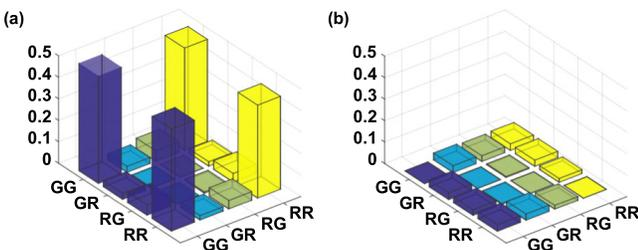
FIG. 4. Reconstructed two-photon OAM state  $\rho_2$ . The real and imaginary parts are shown in (a) and (b), respectively.
