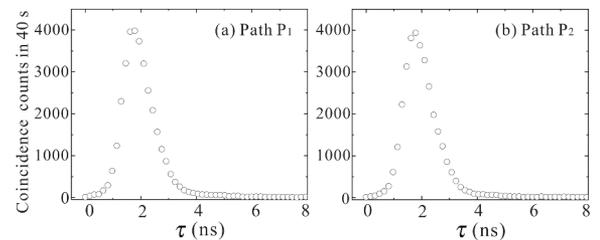
**Fig. 2.** Coincidence counts are measured with 40 s collection time for path 1 (2) when path 2 (1) is blocked.  $\tau$  represents the relative time delay between anti-Stokes photons and Stokes photons. The cross-correlation functions for both paths are  $250 \pm 16$ , which violate the Cauchy-Schwarz inequality by a factor of  $(1.56 \pm 0.39) \times 10^4$ , indicating the high nonclassicality of the biphoton source. The biphoton waveform likeness between (a) and (b) is 98.8%.
